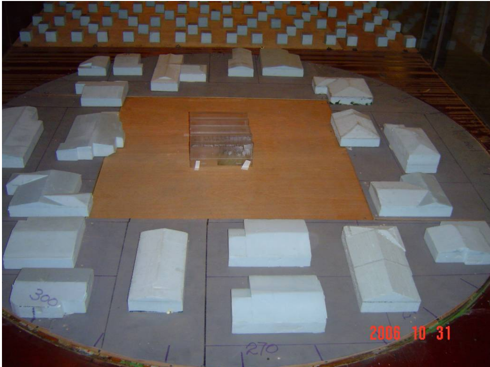
Figure 3.7 Test Model with Surrounding Residential Houses
